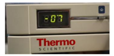
Figure 7-2: Correction value of -0.7 °C shown on display
