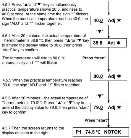
After Temperature calibration, the temperature displayed is the same as the practical temperature of block.
