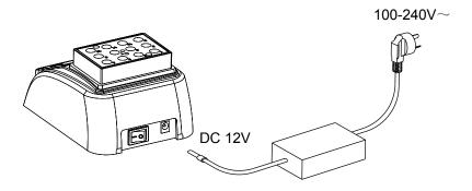
1.3.3 Power on the main switch. The incubator is ready to operate when the display becomes visible.
