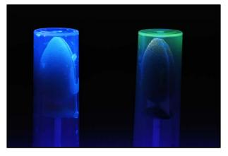
4. For confirmation of *Listeria* spp., examine the bottom of an inverted polypropylene tube for a green fluorescence using a UV lamp at  $365 \, \mathrm{nm}$ . Observe only the plastic tube for fluorescence, not the liquid.
