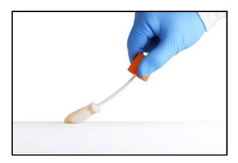
1. Aseptically remove the pre-moistened EnviroMax® Environmental Sampling Swab (Cat. no. 2588050PF) from the container and swab the surface according to the sampling plan.
