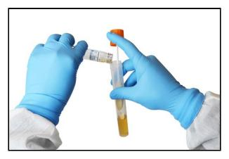
2. Return the EnviroMax® Environmental Sampling Swab to its container and aseptically pour all the contents of the Pathfinder<sup>TM</sup> Listeria Broth tube into the swab container. Incubate tubes at 35-37°C for 30-48hr with the sponge submerged.
