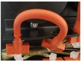
**NOTE**: It is recommended to replace one tube at a time from left to right to keep correct clear elbow connection placement.
