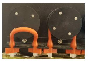
14.2.7. When the orange pump tube is off the roller, pull the tube from the bracket.
