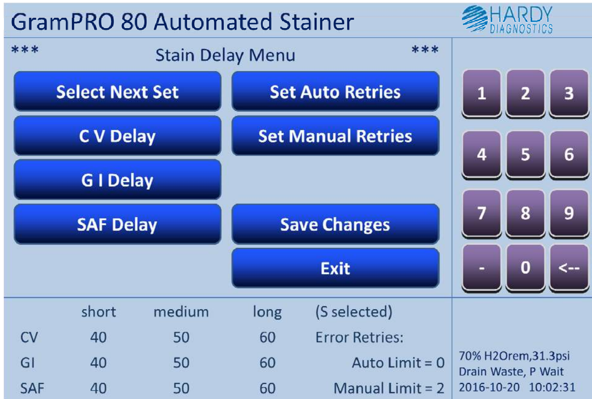
Figure 11.4.1 – Stain Delays Menu
