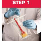
Remove the tear-off strip and carefully take the sani-stick by the handle.
