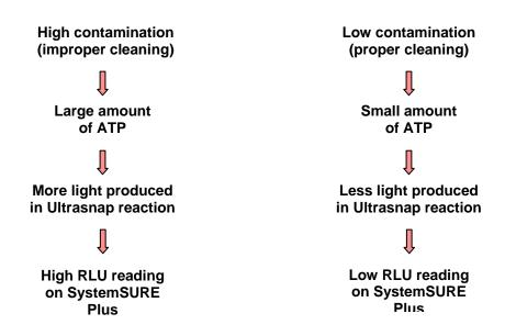
The RLU reading is directly proportional to the amount of ATP collected from the sample. A high RLU reading indicates a large amount of ATP at the test location. This in turn indicates improper cleaning and the presence of contaminants.
