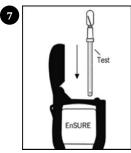
7. Insert device into EnSURE and press OK to initiate measurement.
