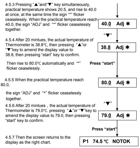
After Temperature calibration, the temperature displayed is the same with the practical temperature of block.
