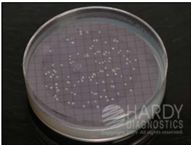
Escherichia coli (ATCC® 25922) filtered through a black membrane (Cat. no. A045R047A) and growing on m-HPC Agar (Cat. no. G95). Incubated aerobically for 24 hours at 35°C.
