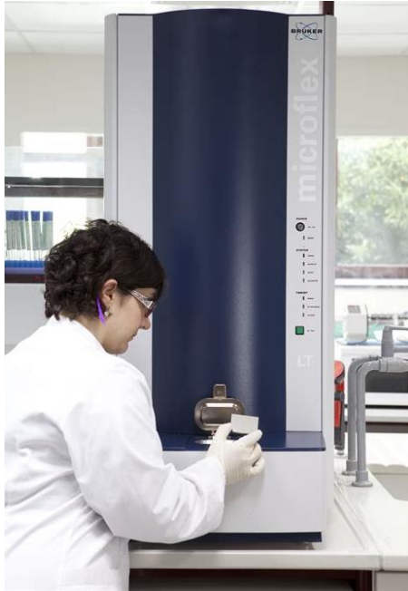
Figure 3: The MALDI-TOF mass spectrometer can be instrumental in the identification of C. auris .
